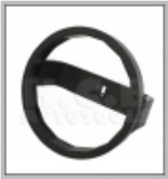
H.C.B-A2018-13 ISUZU/ HINO 17 TONS OIL FILTER WRENCH (EURO 4) (Dr. 1/2", 16 POINTS, 118 mm)
